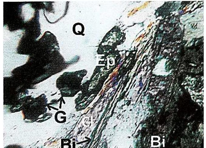
Figure 8. Quartz-feldspar schist with biotite and muscovite (x 2550; N+; original)
