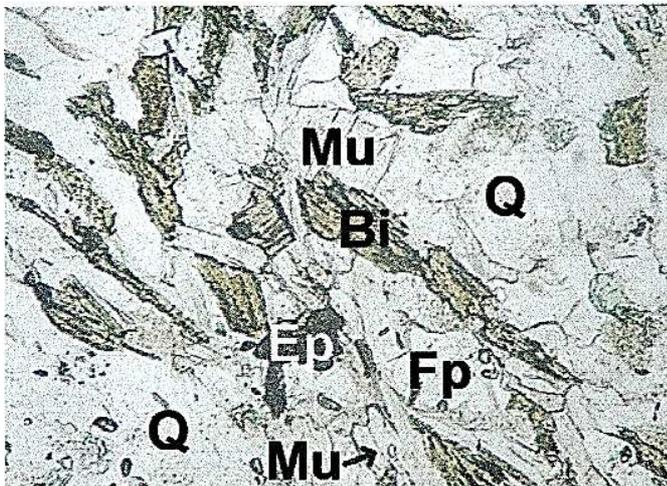
Figure 7. Quartz-feldspar schist with biotite and muscovite (x 257; N II; N II = normal light image; original)
