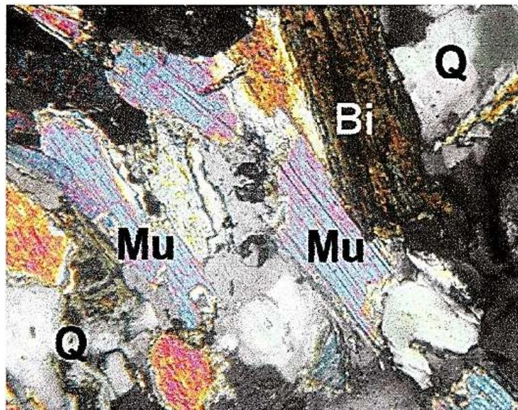
Figure 11. Quartz-feldspar schist with biotite and muscovite (X 509; N+; original)
