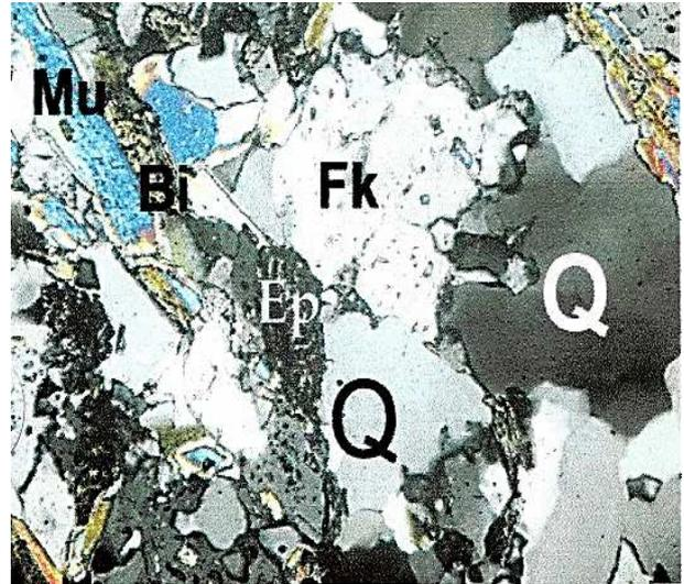
Figure 6. Quartz-feldspar schist with biotite and muscovite (x 257; N+; original)
