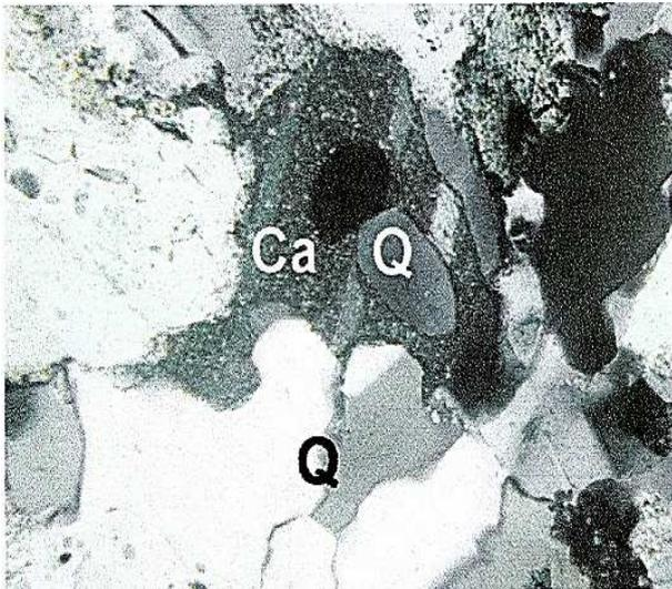
Figure 5. Quartz-feldspar schist with biotite and muscovite (x 509; N+; original)
