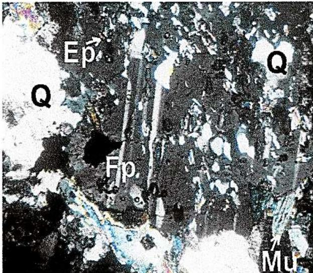
Figure 9. Quartz-feldspar schist with biotite and muscovite (x 257; N+; original)
