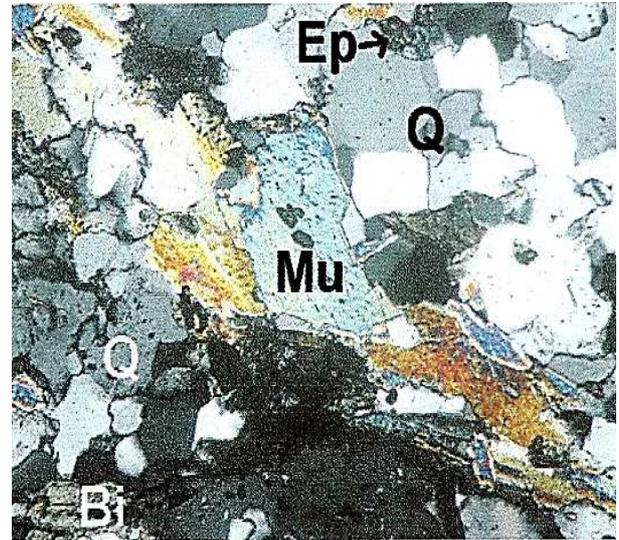
Figure 10. Quartz feldspar schist with biotite and muscovite (x 257; N+; original)
