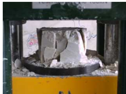
Figure 5. Cubic broken sample to the uniaxial compression test (limestone)
