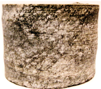
Figure 4. Cylindrical test specimens after the freezing-thawing cycles (schist)
