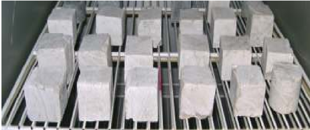
Figure 2. Samples made of the klasts in the limestone scree according to the standards
