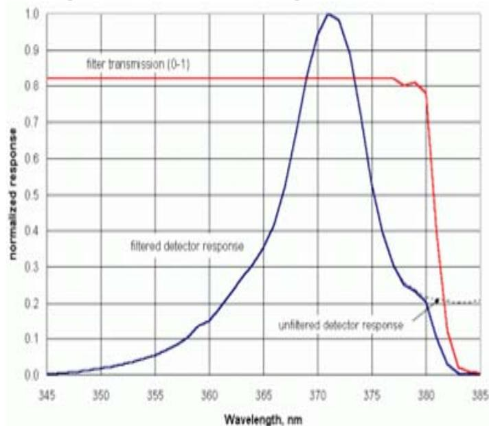
Figure 6. Spectral response of an unfiltered blue LED detector.
