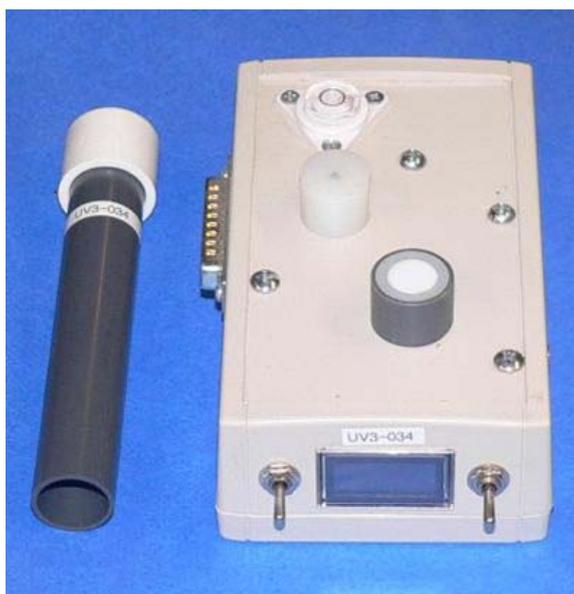
Figure 8. GLOBE/GSFC UV - A radiometer and Sun photometer.
