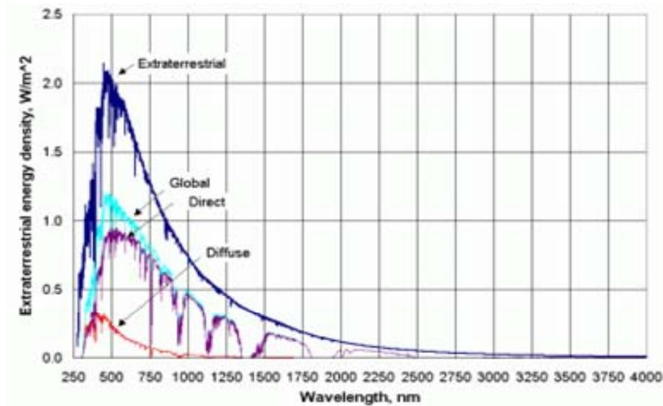
**Figure 1. Direct, diffuse and total insolation for a standard atmosphere with relative air mass of 1.5 (Birds, Riordan, 1994)**
