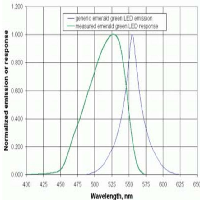
*Figure 5. Generic emerald green LED emission compared to measured spectral response. (Mims, 1992)*
