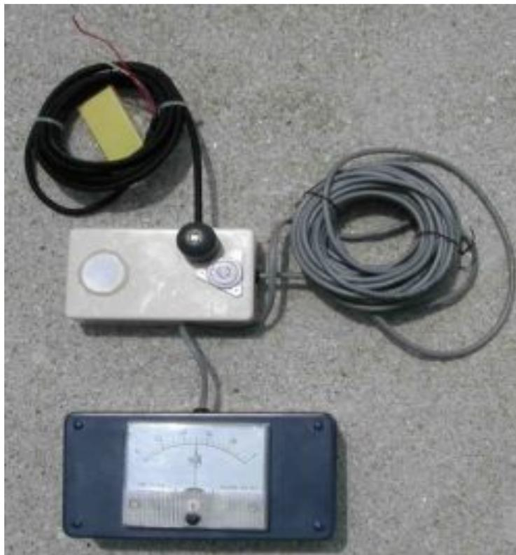
*Figure 4. A solar-cell based pyranometer with an analog microammeter used for calibration (King and Myers, 1997)*
